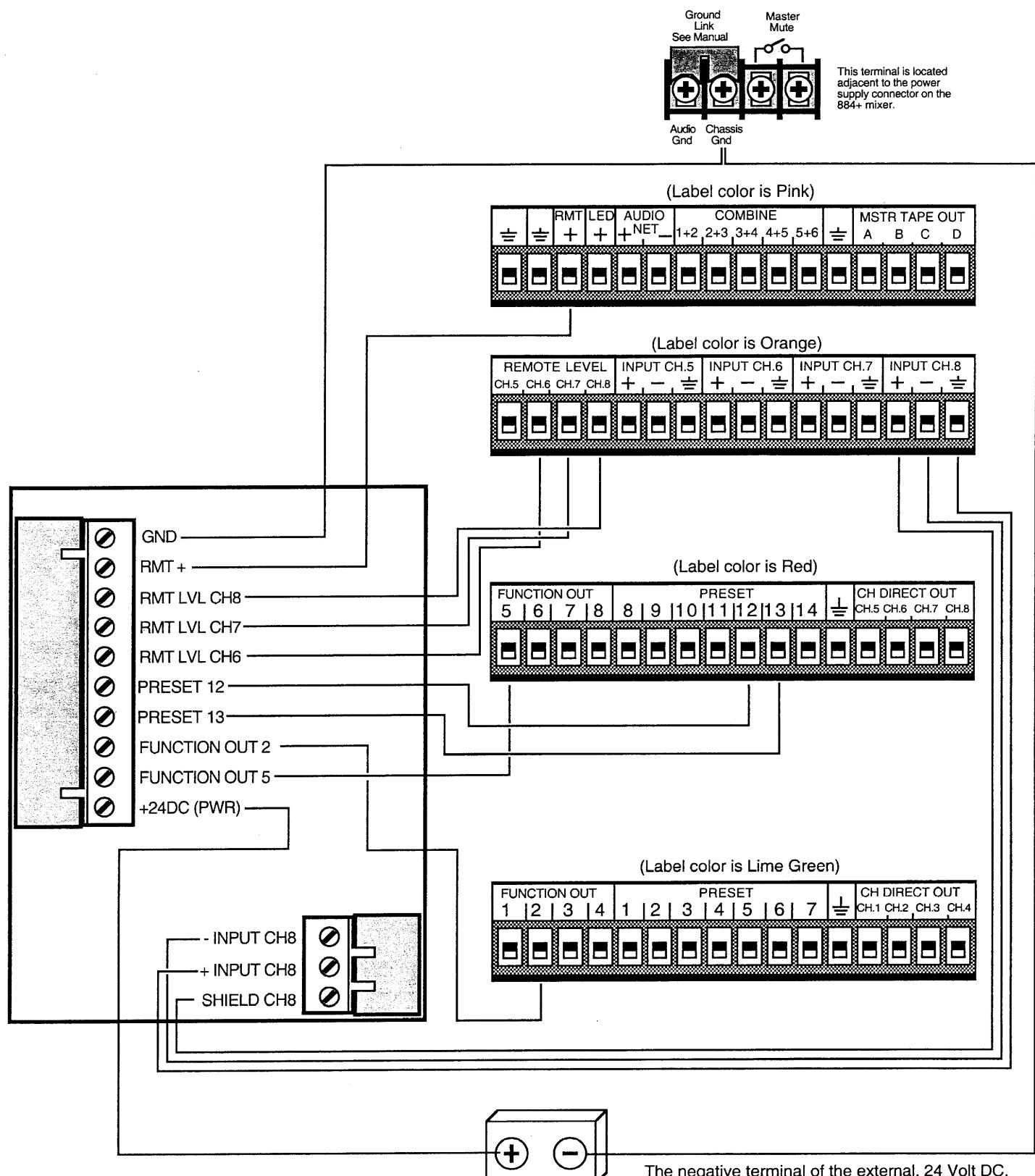
The negative terminal of the external, 24 Volt DC, power supply must be connected to the "Chassis Gnd" terminal of the mixer. DO NOT CONNECT the power supply ground to any other terminal on the 884+.
