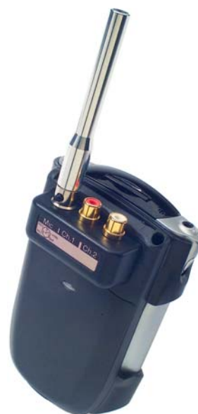
Fig.1: The Ivie Technologies IE-33 turns a compatible PDA into a powerful audio analyzer. The PDA is inserted into a special jacket that includes mike and line inputs, preamp, A/D converter, and battery-management firmware. Also included is a Type II microphone.
