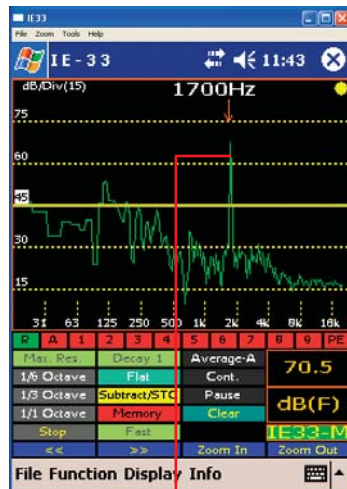
Fig.3: The Frequency Detect option identifies the frequency with the highest SPL.
