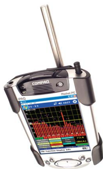
Fig.1: The Ivie Technologies IE-33 turns a compatible PDA into a powerful audio analyzer. The PDA is inserted into a special jacket that includes mike and line inputs, preamp, A/D converter, and battery-management firmware. Also included is a Type II microphone.
