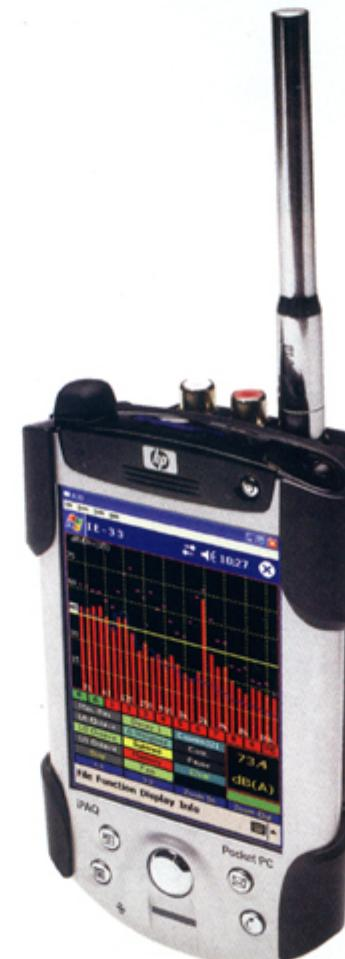
domain capabilities. But I realized that multi-channel simultaneous digital conversion and calculation is likely not realistic given the size, battery power and hardware limitations of today's handheld PDAs. Resigned to live in the real world, the high-resolution RTA and SPL functionality can do a lot of work that could not be imagined with today's rack-mount RTA offerings.
