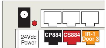
Wiring between the CP-884C and the 884-IF is accomplished using a conventional CAT-5 cable conforming to the EIA 568B standard.
