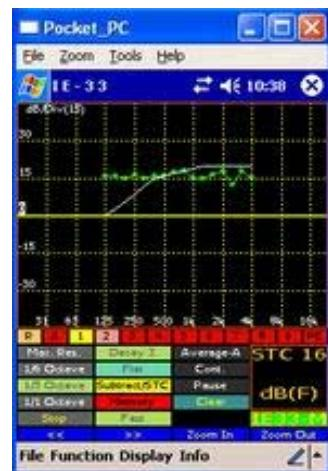
The IE-33 runs NIC contour calculations and shows NIC display PLUS calculating the appropriate correct NIC number.
